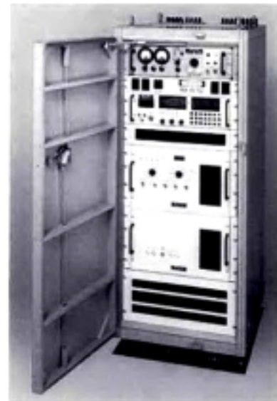
AN/URC-119(V) configured for shipboard use
